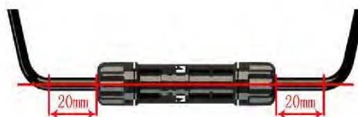
Right way for the cable
