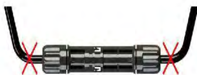
Wrong way for the cable
